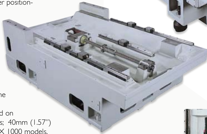
GX 600 and GX 1000 Y-axis guideways shown
