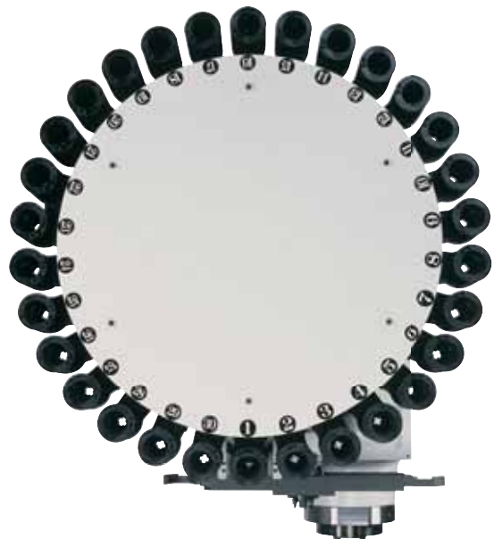
30-tool Swing-arm ATC shown
