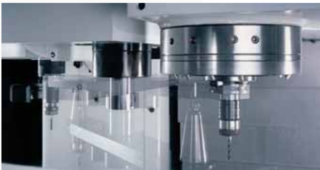
48-tool Swing-arm ATC shown
