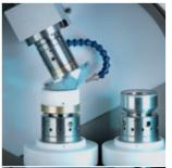
The SLP 120 E is capable of multistep polishing with individually controlled CNC parameters.
